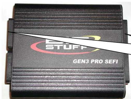
The header connector will be marked "DAE" to indicate where to connect the DAE harness to.
